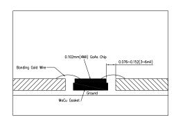
Note: Microstrip substrates should located as close to the die as possible in order to minimize bond wire length.
